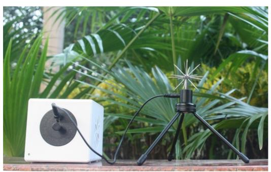
Pic. 1. Connection of the Sputnik sensor to the Bio-Well device.
